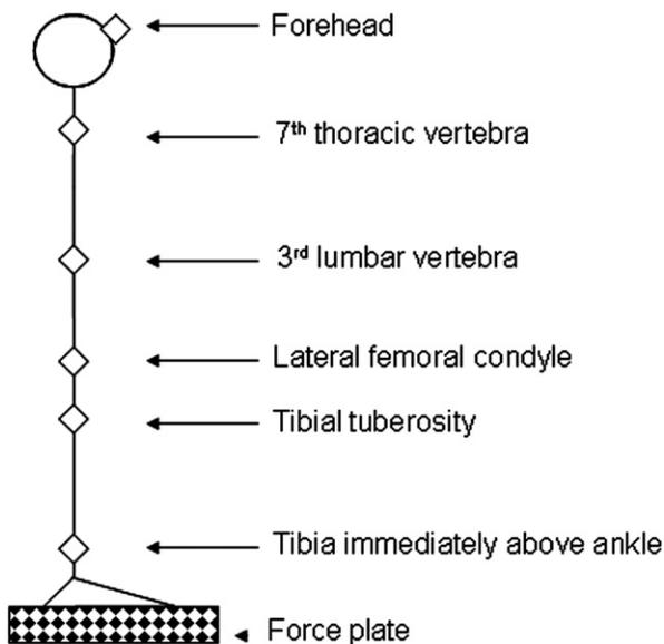
Fig. 1. Schematic of accelerometer-placement sites.
