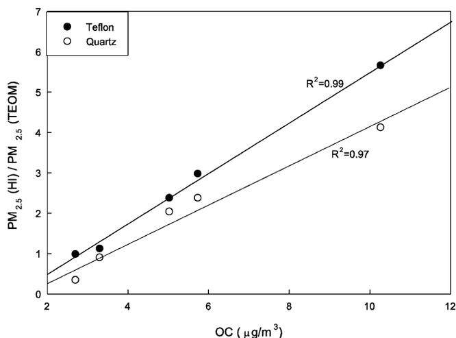
**Figure 3.** Ratio of PM<sub>2.5</sub> measured by the HI (Teflon and quartz) and TEOM as a function of OC levels at all sites.
