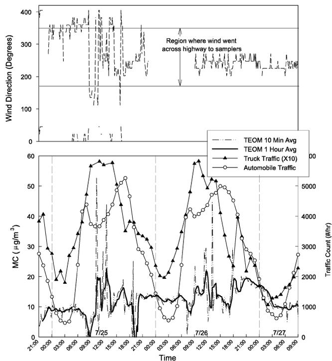
**Figure 4.** Automobile and heavy-duty truck traffic density and average mass concentrations (TEOM), versus time, at the Findlay sampling site (25 and 26 July 2002). The two solid lines in the wind direction figure indicate the time when wind was directed from the highway to the sampling location.
