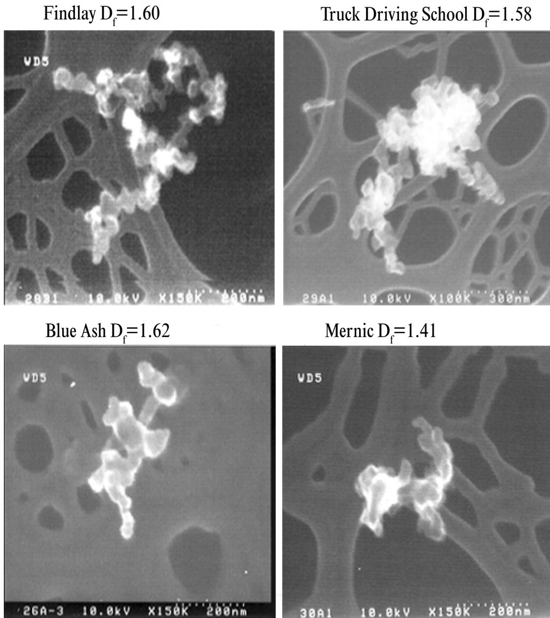
**Figure 5.** SEM images of aggregates collected at the four sites. Also listed are the average 2D fractal dimensions.
