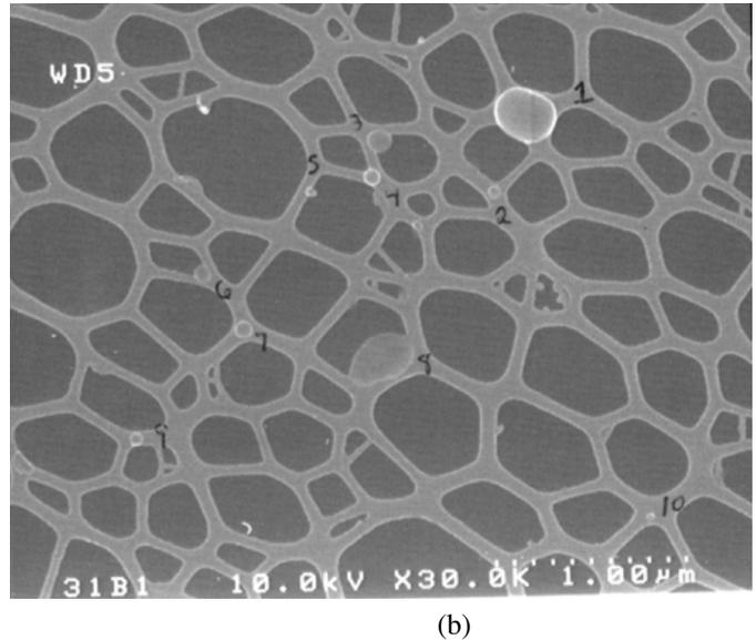
**Figure 7.** (a) Size distributions measured with the DMA at Mernic on 31 July 2002. (b) Electron micrograph of numerous small spheres collected at the Mernic site.
