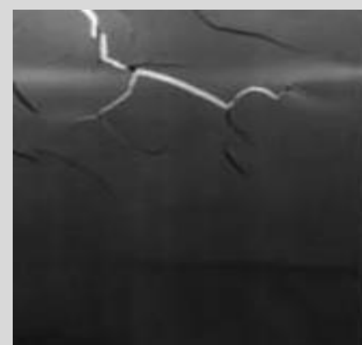
Cracked lead shield; Diagn. Interv. Radiol. 2012; 18:147-152
